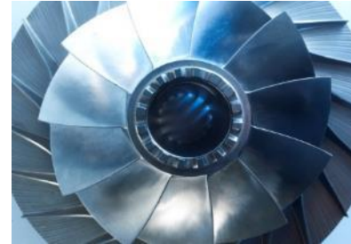
Helicopter engine impeller (Inconel)
